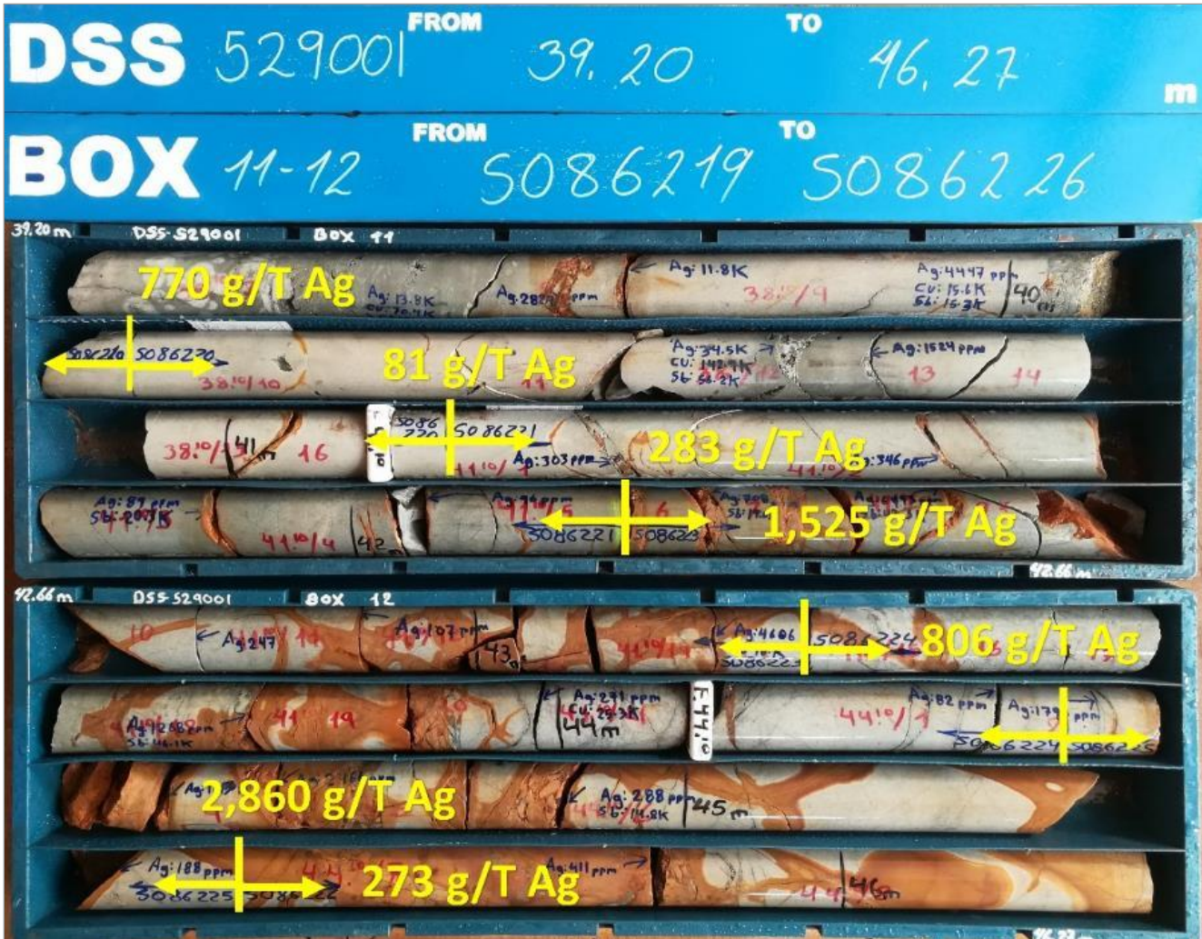
Figure 7.16 Transition material in core
